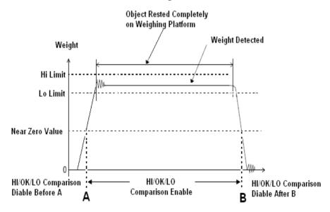
After Hi, Lo limits and near zero value have been entered, this instrument is ready for dynamic checking.
